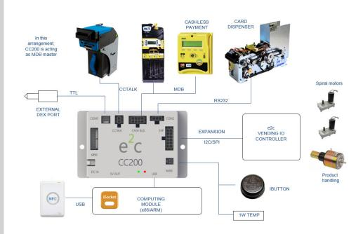
The CC200 smart device hub allows combinations of complex peripheral - from any manufacturer - within the same machine! This allows manufacturers to take the best of breed payment devices to create bespoke payment solutions.
